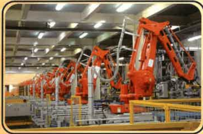
Figure 4: Integrated robotic palletizing system for multiple production line
