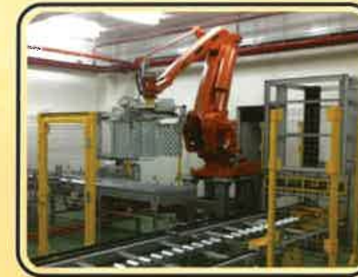
Figure 6: Palletising robot with gripper
