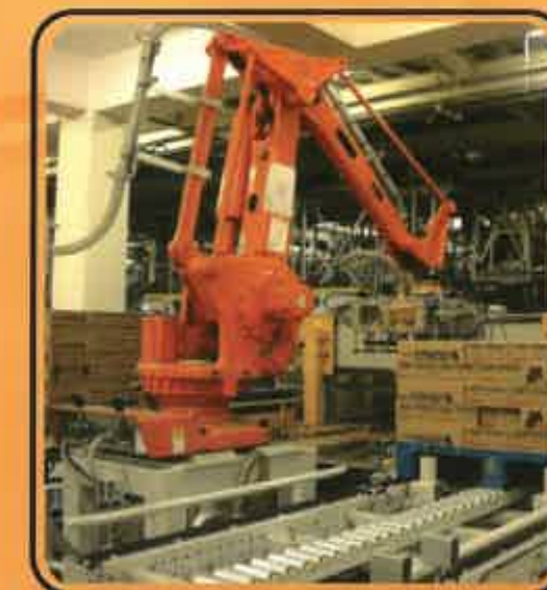
Figure 7: Palletising robot with suction mechanism
