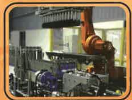
Figure 2: Bottle Pick and Place to carton box
