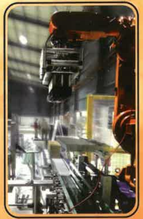
Figure 3: Bottle Pick and Place to carton box
